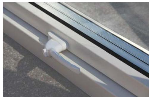
A multi-layered deep-impregnated window, the bottom sash is protected with an aluminium glazing bead. To reduce heat loss at the edge of the glass, we recommend using an insulated glazing that has SWS (plastic) spacers rather than the traditional metal.
